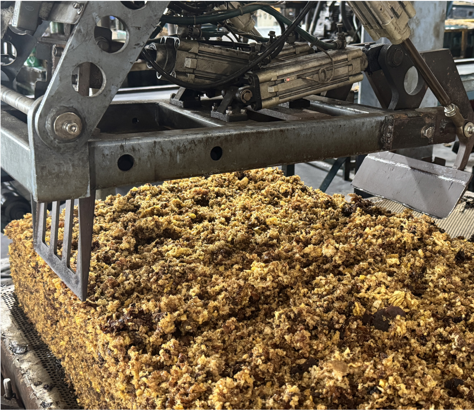
搭载 AI 算法的生产线自动转运块状橡胶半成品，完成工位间流转 An AI-powered production line automatically transfers semi-finished rubber blocks between workstations.
